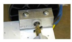
Too much overhang (remember Saint-Venant!). Consider the use of an outrigger bearing, or mount the wheel on a properly supported shaft and drive the shaft with the motor using a coupling
