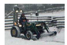
Nick Powley obtained 4WD by cutting grooves in his wheels and using rubber bands as drive belts...
