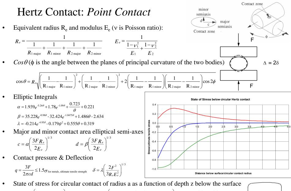
$$\sigma_{z}(z) = q \left(-1 + \frac{z^{3}}{\left(a^{2} + z^{2}\right)^{1.5}}\right) \qquad \sigma_{r}(z) = \sigma_{\theta}(z) = \frac{q}{2} \left(-(1 + 2\nu) + \frac{2(1 + \nu)z}{\sqrt{a^{2} + z^{2}}} - \frac{z^{3}}{\left(a^{2} + z^{2}\right)^{1.5}}\right) \quad \tau(z) = \frac{\sigma_{\theta}(z) - \sigma_{z}(z)}{2}$$
