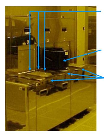
Kinematic coupling pins on loadport based on SEMI E57 standard
