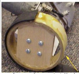
Improper surface preparation (rubber should be clean and rough), and the rubber should have been scarf joined
