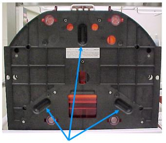
Mating kinematic coupling grooves on the FOUP, permitting precise alignment on load ports, so robots can precisely access 300 mm wafers
